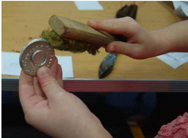
Polishing an object cast from tin
